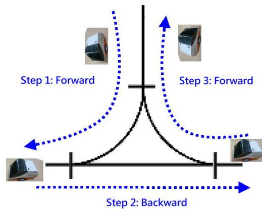
Figure 2: Three steps for the train to turn round
